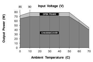
Derating requirements - Derate from 100% load at 50° C to 50% load at 70° C. - Derate from 100% load at 90 Vin to 90% load at 85 Vin - Derate 10% with chassis and cover.
