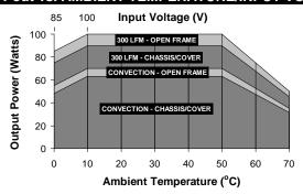
Derating requirements – Chart above applies to models 1003 thru 1008 only. 100 Watts 300 LFM forced air, open frame. 70 Watts convection cooled open frame. Derate 10% with chassis and cover. Derate 1.0 Wout / 1 Vin below 100 Vin and between 100 Vin and 85 Vin. Use larger of the two deratings when using chassis/cover below 100 Vin. Derate output power linearly to 50% between 50° and 70° C
